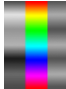
Figure 4.3.1: Desaturation of spectral gradient with luminance (left) and mathematical average (right)
