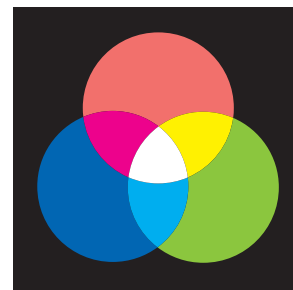
Fig. 2.1.1.1: Projection of three lamps with the colors Red, Green and Blue onto a wall in a dark room
